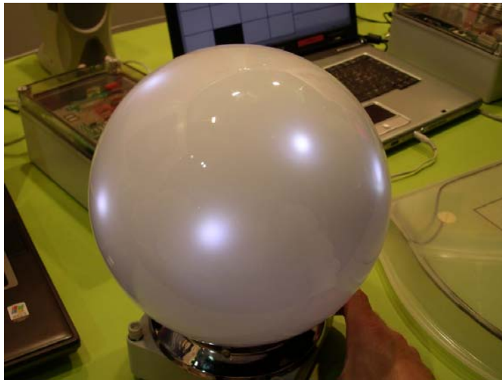
Fig. 4. The light globe with LED's placed under the surface and indicating the position of sensitive spots.
