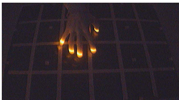
Fig. 3. Image seen by the camera. Visible light is filtered out using a 800nm pass filter.
